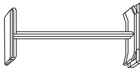
Figure 2.6.H Snaplok™ 406 Sheet Ending Tool Incorporating Ender and Down-turner
